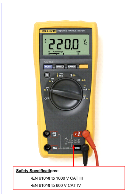
Figure 5: Identifying the Insulation Category of Test Equipment
